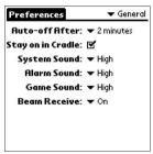
2 Tap the arrow ▼ next to Auto-off after and then select the desired time setting for the automatic shut-off feature.
